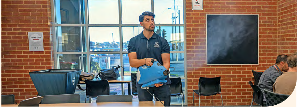
Image: Burnet’s Loukas Tsigaras calibrates rooms at Northcote Library as part of the PCIA project. Loukas and fellow engineers from Melbourne University gather baseline data on particle dispersion in the rooms before air filters are installed.
